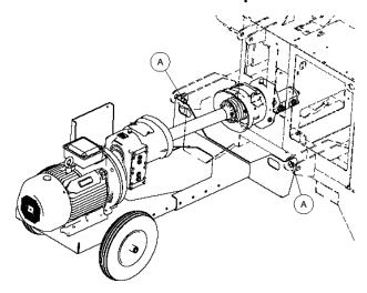
The EP75 and EP110 have wheels and can be easily moved by driving them like a wheelbarrow. They are attached to the firewood processor using drawbar bolts illustrated with A.
